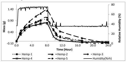
Fig. 18. Kinetics of moisture buffer of hemp insulations during the final cycle.
