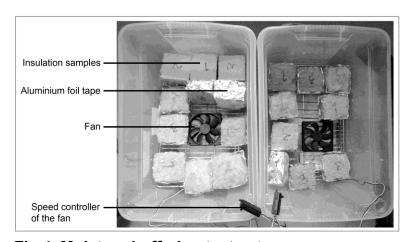
Fig.4. Moisture buffering test setup.
