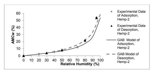
Fig. 8. Adsorption-desorption isotherm (AMCw) of Hemp-2 with GAB fit.
