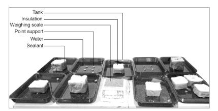
Fig. 5. Setup for assessing water absorption coefficient (A value).
