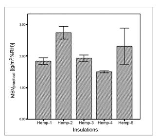
Fig. 17. Practical moisture buffer value of the insulations with 1 standard deviation.
