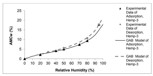
Fig. 9. Adsorption-desorption isotherm (AMCw) of Hemp-3 with GAB fit.
