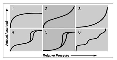
Fig. 2. IUPAC classification of adsorption isotherms.
