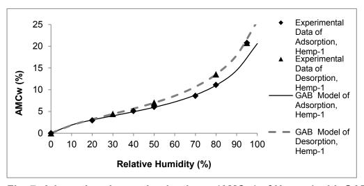
Fig. 7. Adsorption-desorption isotherm (AMCw) of Hemp-1 with GAB fit.
