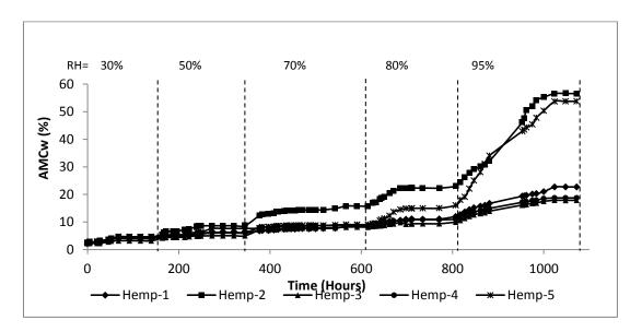
Fig. 13. Adsorption kinetics of the hemp insulations.
