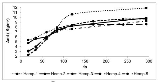
Fig. 15.  $\Delta m_t$  versus  $\sqrt{s}$  plot for Hemp-1, Hemp-2, Hemp-3, Hemp-4 and Hemp-5 insulations (average values of 3 samples).
