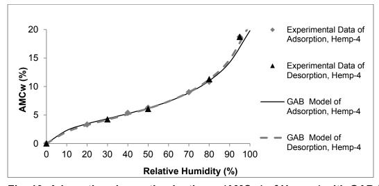
Fig. 10. Adsorption-desorption isotherm (AMCw) of Hemp-4 with GAB fit
