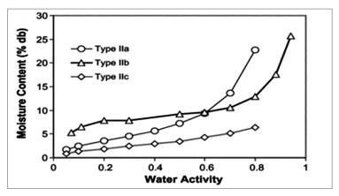
Fig. 12. Modified classification of type II isotherms [20].
