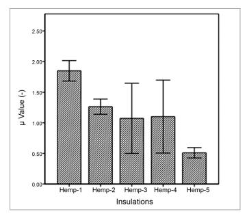
Fig. 14. Vapour diffusion resistance (  $\mu$  value) factor of the hemp insulation materials during the wet cup test with 1 standard deviation.
