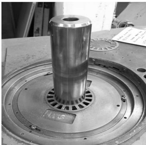
**Fig. 2.46.** Slot liner insertion machine.
