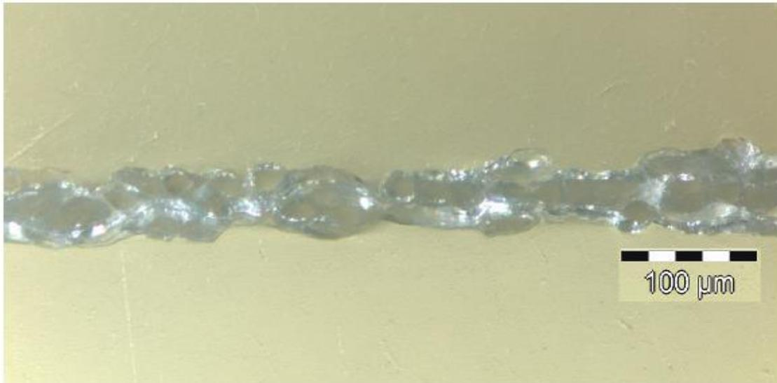
**Fig. 6.16.** Paper wall insulation material without resin impregnation (DuPont, 2012).
