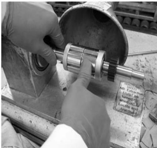
**Fig. 2.74.** Finalizing the permanent magnet insertion manufacturing process.
