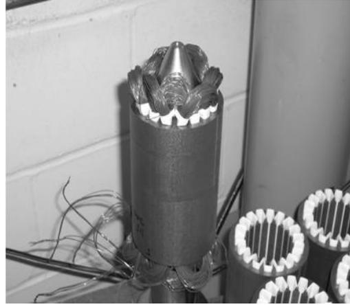
**Fig. 2.53.** Complete winding inserted.
